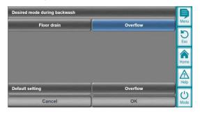
An info text (at the bottom of the menu) summarizes the result of the current configuration, e.g. "During a backwash, suction is taken out of the gutter tank"
