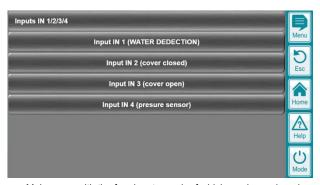
Main menu with the four inputs, each of which can be assigned a label
