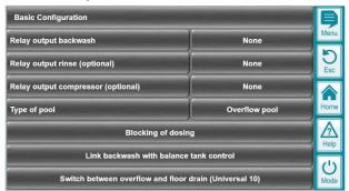
Assignment of the relay outputs used
